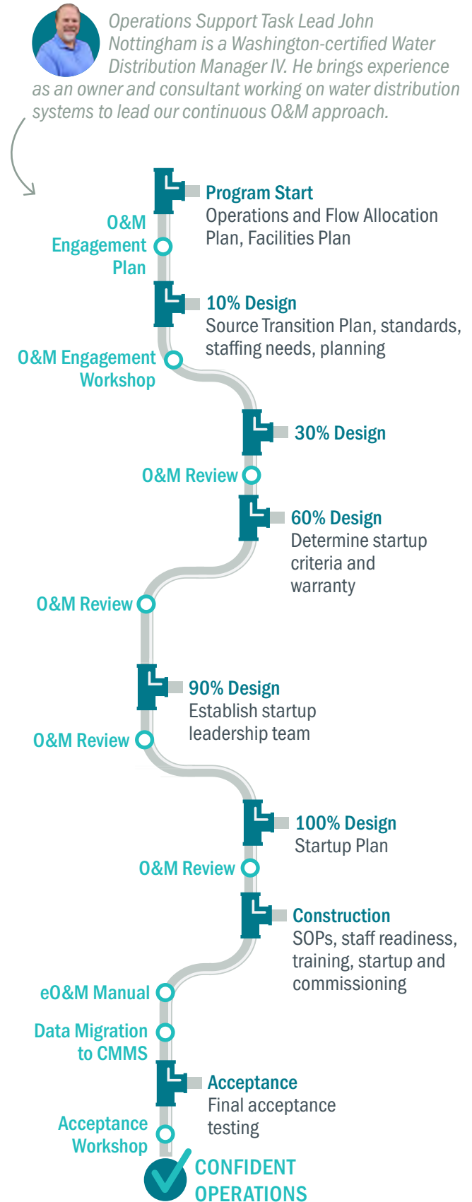
Figure 5.3 // Continual O&M engagement lays the foundation for reliable, maintainable, and long-lasting assets.
