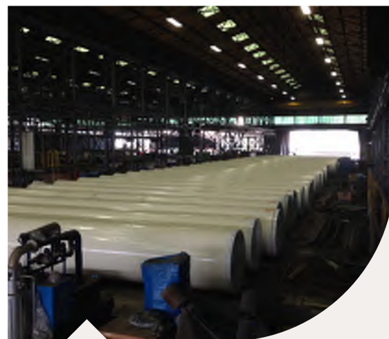
Northwest Pipe facility, Portland, OR. Coated and lined steel pipe for WWSP.
